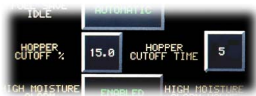
The Moisture Mirror includes a hopper cutoff function to immediately close moist air valves when wet cotton enters the gin.
