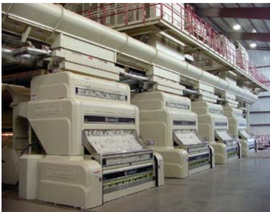
A new style of double-entry hoppers places the valves on the side and avoids a moist air pipe over the gin apron.
