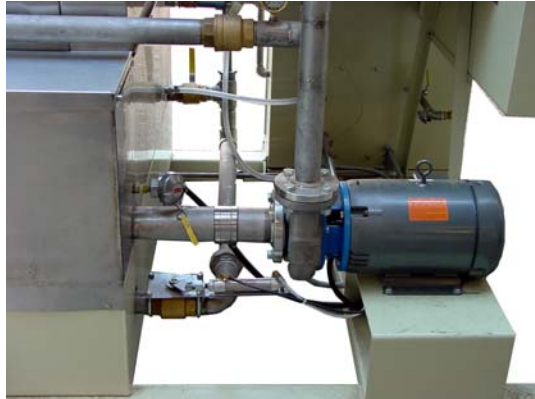
7-1/2 HP cast stainless pump delivers performance
