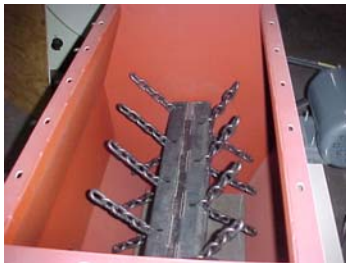
A chain flail located above the Hot Box can disperse wet UNR and stripper cotton for better drying and cleaning.
