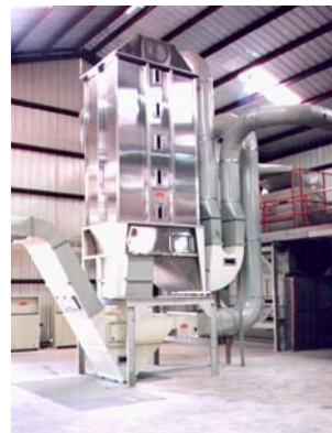
A Fountain Dryer with a collider-rock trap to separate debris with hot air.
