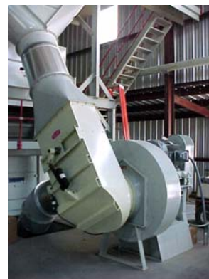
The Electric Banjo can be used on unloading fans or on drying system pull fans to increase operating air volume 30%
