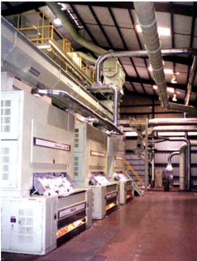
Conditioning Hoppers between the feeders and conveyor distributor humidify seed cotton to protect staple, reduce short fiber, and improve final moisture restoration.
