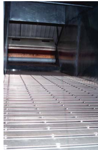
The batt of lint cotton floats to the press on a bed of humid air provided by this stainless steel Lint Slide Grid.
