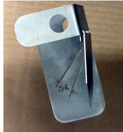
The swinging vane should float between the two lines in the area marked "OK"
